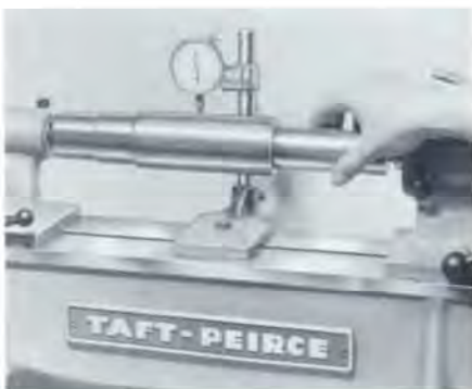
Rotating work against dial indicator to determine runout.
