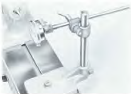
Mounting, Bracket, and .0001" Dial Indicator are useful Bench Center accessories available at slight extra cost.
