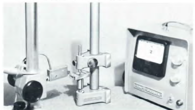
To indicate face runout, stand the Instrument Bench Center vertically on precision ground headstock pads. Surface plate is Taft-Peirce No. 9213.
