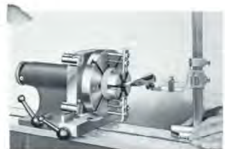
Checking the accuracy of a female spline gage mounted on Sine Bar Indexing Head by means of auxiliary circular face plate. Gage Blocks placed on the base reference bar provide a highly accurate means of setting any desired index angle.
