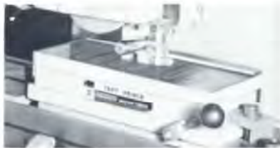
Grinding flat on a cylindrical workpiece held in No. 9129 V-Block. Machine is the Taft-Peirce No. 1 Precision Surface Grinder.
