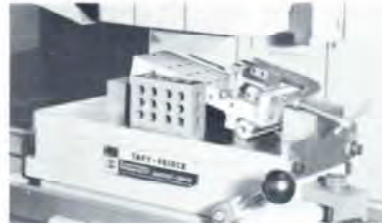
5" Sine Block makes fast set-up for grinding precise angle on end of shaft. V-Block is Taft-Peirce No. 9129.
