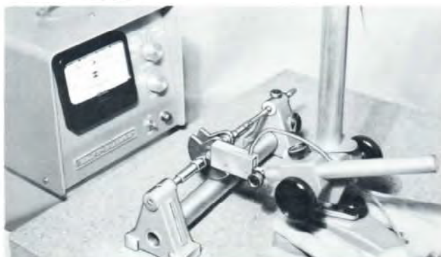
Checking concentricity of miniature crankshaft after O.D. grinding operation, using the Taft-Peirce Versachek Electronic Gage.
