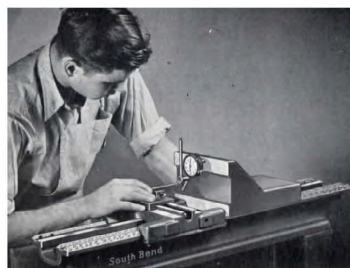
Fig. 1. Testing the Saddle Cross Slide Dovetail for Squareness with V-Ways of the Lathe Bed
