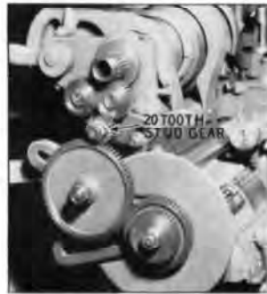
Fig. 36. Model A Lathe set up for cutting threads 8 to 224 per inch
