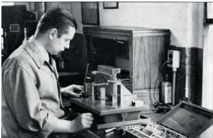
Fig. 6. Below—Checking a Fixture
