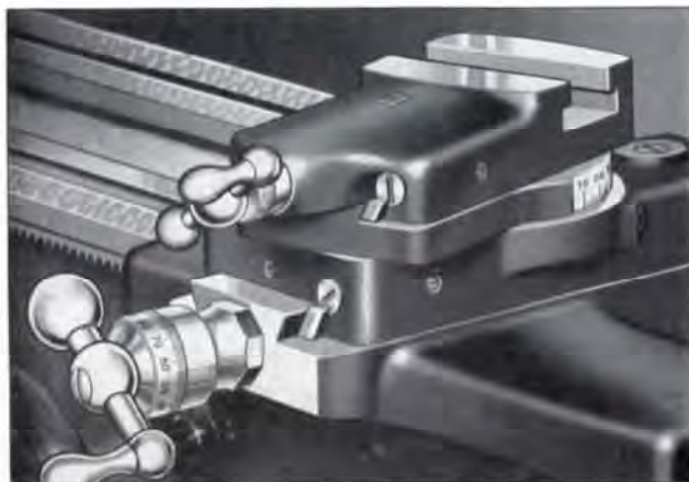
Fig. 20. Close-up Showing Adjustable Tapered Gibs Used on Compound Rest Base and Top Dovetails of 10-inch and Larger South Bend Lathes
