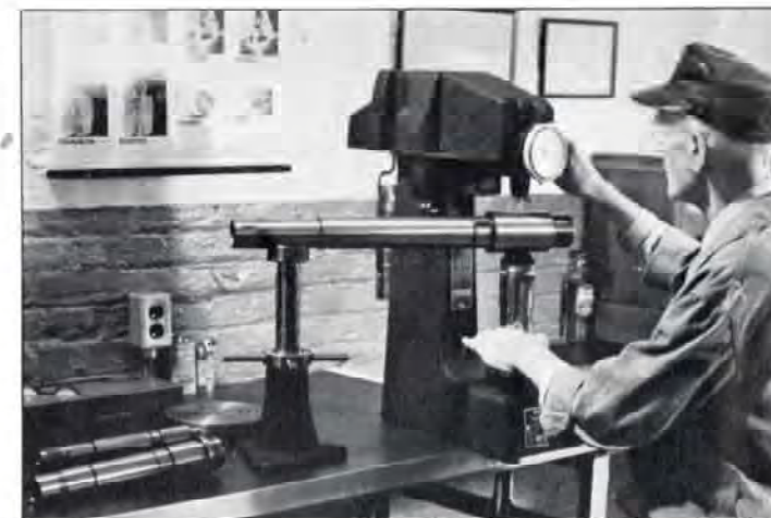
Fig. 4. Testing the Hardness of a Carburized Headstock Spindle Bearing Surface
