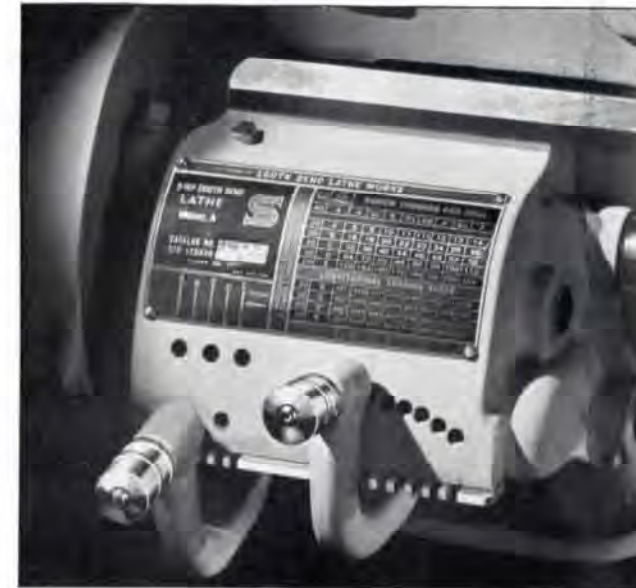
Fig. 34. Quick Change Gear Box Supplied on all Model A 9-inch South Bend Lathes
