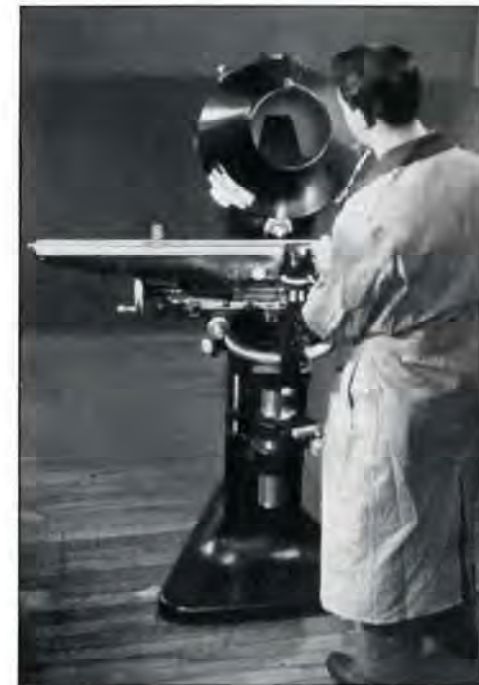
Fig. 7. Inspecting a Screw Thread with an Optical Comparator
