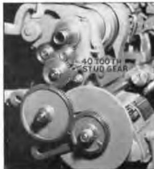
Fig. 35. Model A Lathe set up for cutting threads 4 to 7 per inch
