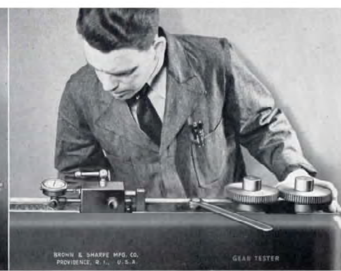
Fig. 3. Testing Gears for Accuracy of Tooth Form, Pitch Diameter, and Concentricity
