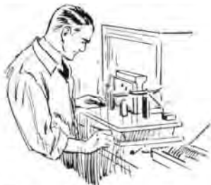
Checking a Fixture with Precision Gauges
