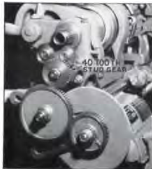
Fig. 2. Model A Lathe set up for cutting threads 4 to 7 per inch
