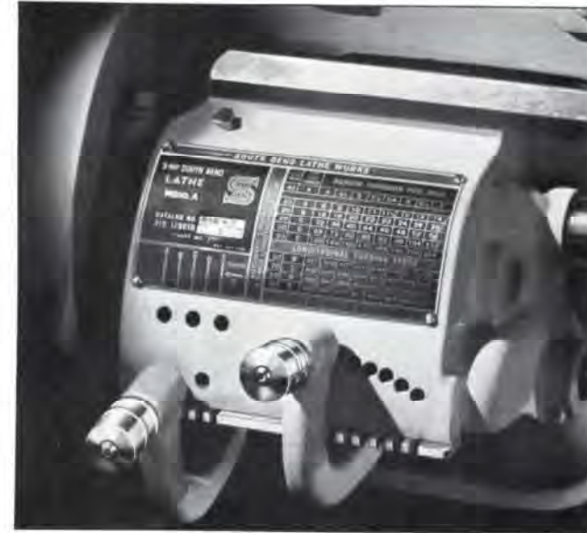
Fig. 1. Quick Change Gear Box Supplied on all Model A 9-inch South Bend Lathes
