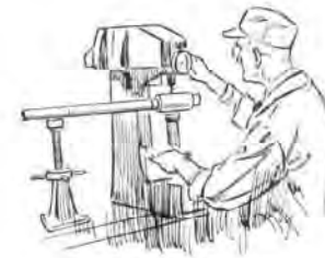
Testing the Hardness of a Carburized Headstock Spindle Bearing Surface
