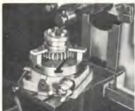
Machining clutch teeth with rotary indexing table.
