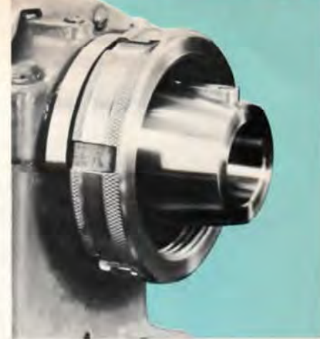
Right — Type L00 Long Taper Key Drive Spindle Nose.
