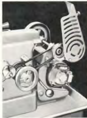
Guards on all belts and pulleys. Quick-acting belt tension release.
