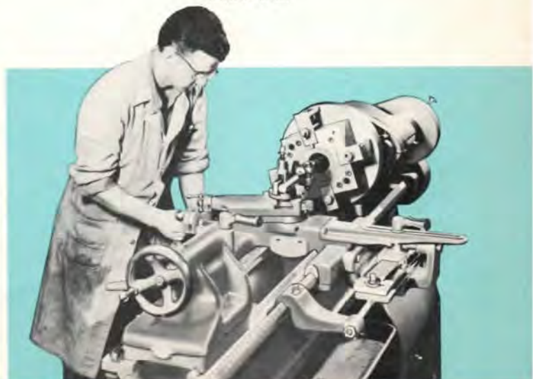
Internal Boring of Mold Section mounted on fixture plate.
