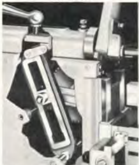
Rocker arm graduated for accurate stroke adjustment.
