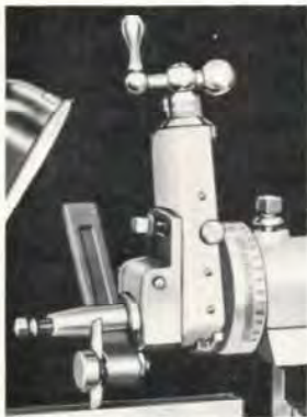
Tool head locks in any position. Rugged clapper box also adjustable.
