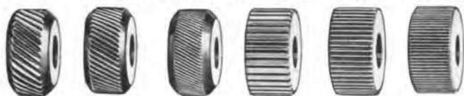
COARSE 14 PITCH MEDIUM 21 PITCH FINE 33 PITCH COARSE 14 PITCH MEDIUM 21 PITCH FINE 33 PITCH
