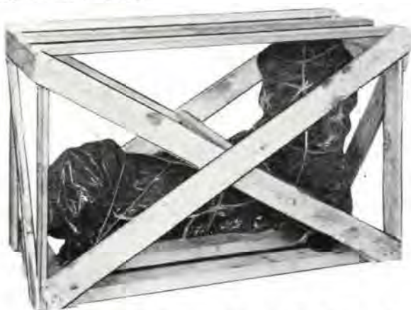
Sheldon Bench Lathe crated for local delivery. In uncrating, first loosen cross braces and uprights at bottom and lift crate off the lathe.
