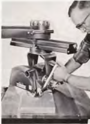
BIG CAPACITIES. Cuts stock up to 3" thick and rips to the center of a 50" panel, with ample table support. In addition, Delta's famous "Turret-Arm" action permits the blade to stay positioned over the table throughout the 360° arm swing. You can even cut left-hand miters and still get full capacity over the table.
