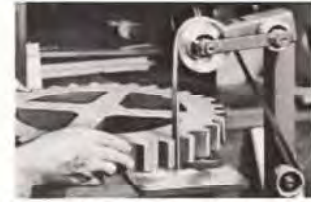
Pattern Shop . . . narrow band gets into small openings . . . finishes patterns rapidly to close tolerances.
