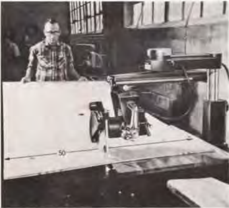
BIG CAPACITIES. Cuts stock up to 3" thick and rips to the center of a 50" panel, with ample table support. In addition, Delta's famous "Turret-Arm" action permits the blade to stay positioned over the table throughout the 360° arm swing. You can even cut left-hand miters and still get full capacity over the table.
