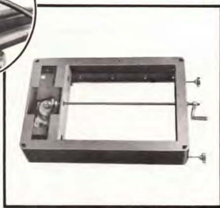
HEAVY, DEEP CHANNEL FRAME CONSTRUCTION. This underside view of the frame shows its rugged, box-type construction that makes it practically distortion proof. This assures continuous alignment of the entire machine, guaranteeing the user trouble-free performance and accuracy year after year.
