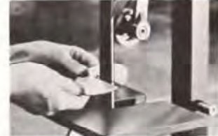
Assembly Department . . . quickly removes sharp edges on metal stampings, even in small openings.
