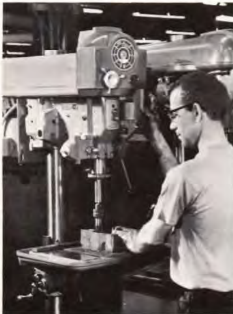
The portability of the New Delta 17" Variable Speed Drill Press permits it to be temporarily placed in a permanent multiple spindle production line to handle an extra operation on a short run part.
