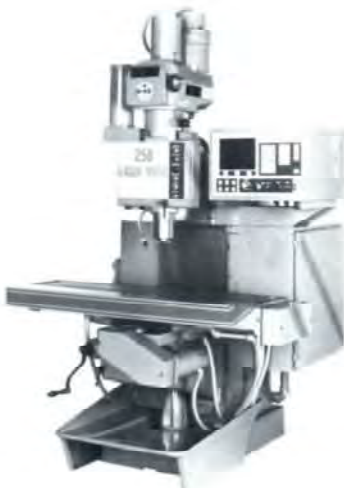
CNC MACHINE shown with air powered draw-bar and CNC Control (Built in California)
