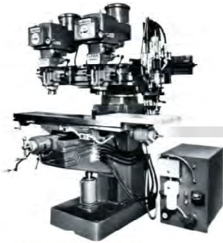
2 AND 3 HEADS T-RAM 3D Tracer Mill w/fluid motors
