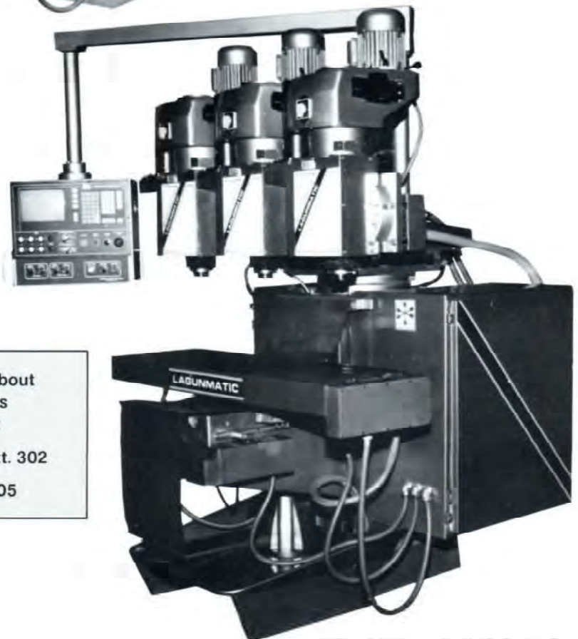
LAGUNMATIC — 3 HEAD CNC MACHINE (Built in California)
