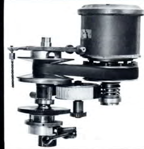
Shown the extra large variable speed pulleys and back gears.
