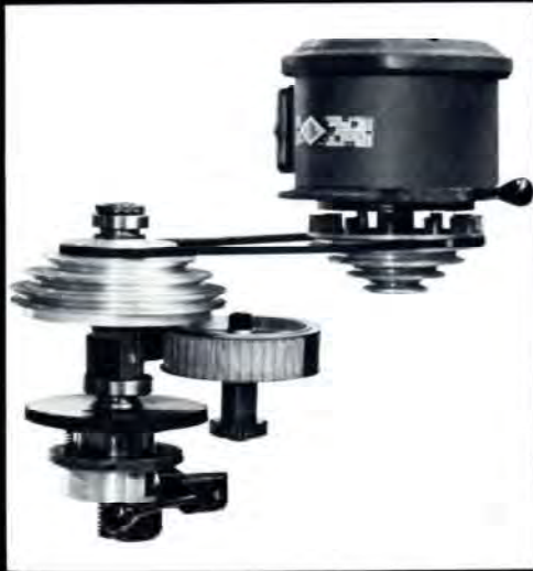
Shown step pulleys and back gear mechanism.
