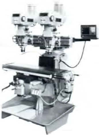
T-RAM 2 HEADS with Feed Motors
