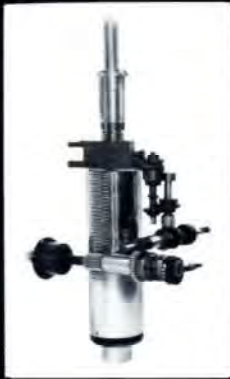
Shown the chrome hardened quill and the ground rack and the counter balanced spindle.
