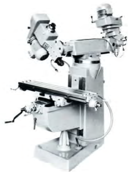
VERTICAL MILLING MACHINE Shown with Slotter Attachment (See page 3)
