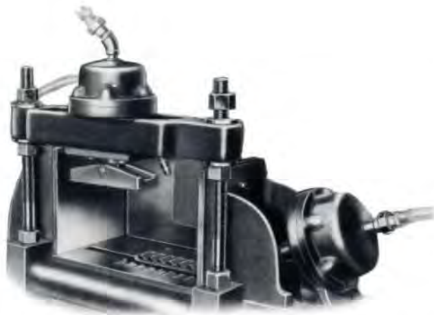
2. Automatic Side and Overhead Hydraulic Chuck on Machine
