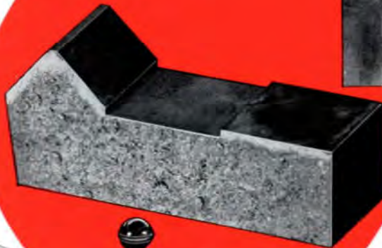
CROSS SECTION AFTER HARDENING
