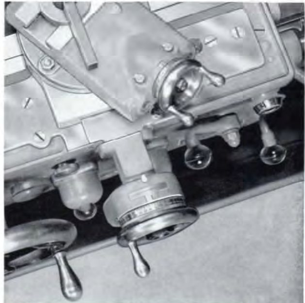
Large Direct-Reading Dials contribute to speed, accuracy and convenience in operation. The easy-to-read graduations give work diameter reductions in thousandths of an inch on the cross slide and on the compound rest.
