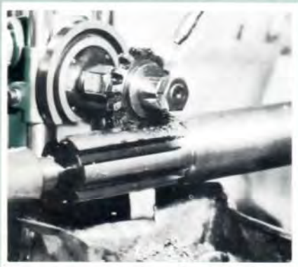
Large keyways can be milled with the Master Unit using end mills or shell end mills working into the side of shaft on center line. Same set-up for milling Pratt & Whitney round end keyways.
