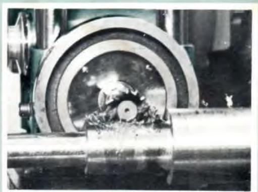
Milling spur gear with a Master Converter in lathe using Master geared Dividing Head in lathe spindle for precision indexing.
