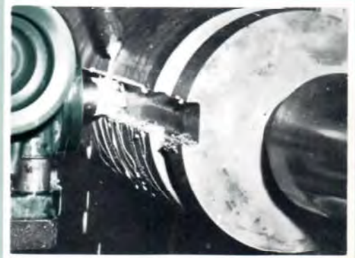
Milling splines, either rebuilding or making new, is profitable with a Master and Dividing head assures accurate indexing. A Master Slotting head does internal splines.
