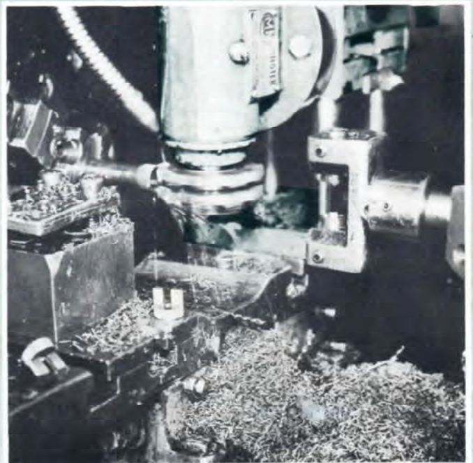
Straddle milling on a turret lathe with Master Model "B" milling attachment completing part in turret. Twelve seconds for \frac{1}{2} " cut on \frac{3}{4} " bar stock.
