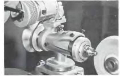
Sharpening a piloted countersink. Cam is adjusted to delicate lift to produce chatterless cutting. Grinding time—
