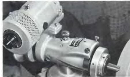
Sharpening a 5/16" tap. Seconds of rotation and the tap is sharp and ready to cut. Grinding time—
