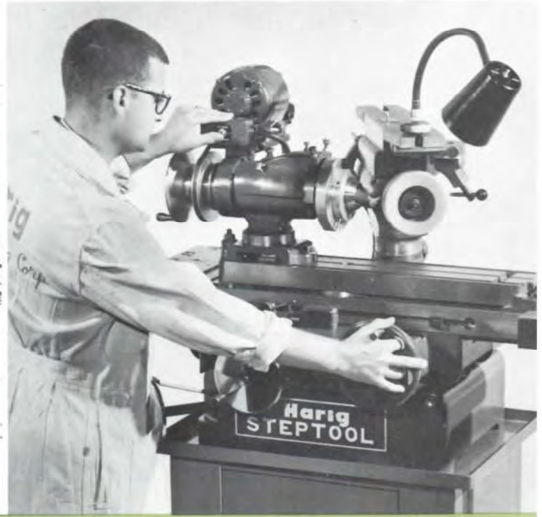
The same simple technique is employed on a 2" drill which is pointed with exceptional accuracy on the large capacity headstock.
