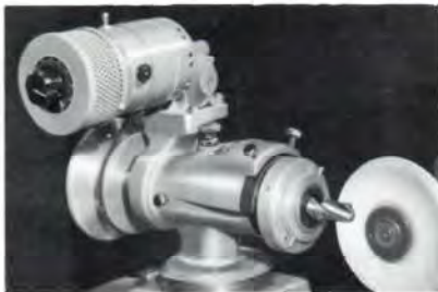
Grinding a 1/4" stepdrill to print. Savings can pay for machine in months. Grinding time—
