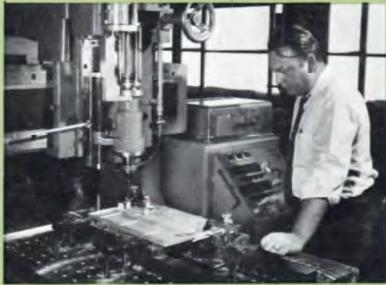
Fred Chelcun, manufacturing engineer at DITTO Inc. observing a helixpoint drill entering a rough casting without prior center drilling.
