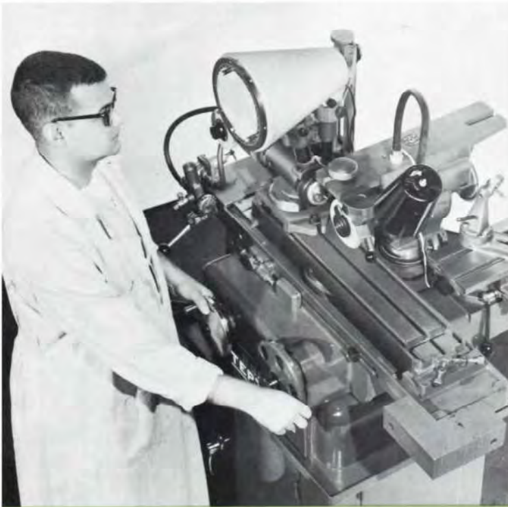
Operator clearly views image of stepdrill on optical comparator. No need to remove tool for inspection.
