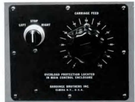
Independent Electrical Variable Feeds
