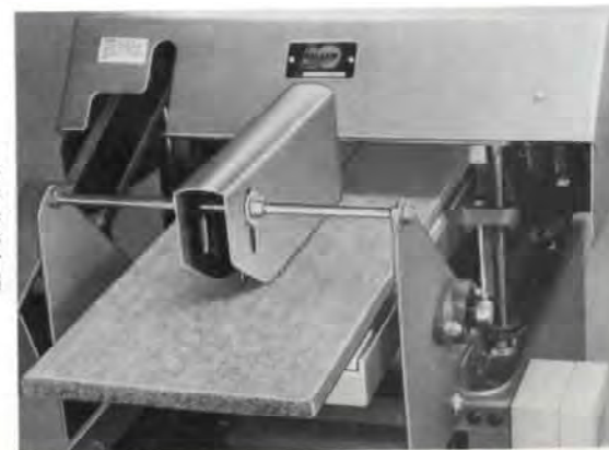
FACE MOLDING — This board is emerging sawed to width, planed to the desired thickness and molded for baseboard use, all with power feed.
