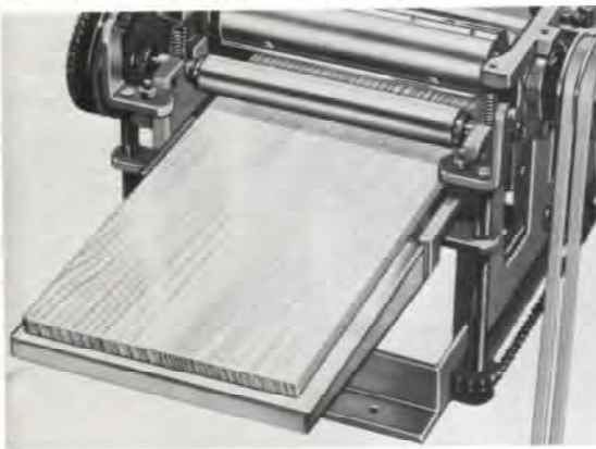
PLANING — Cutterhead uses three planer knives to surface stock up to 12¼-in. wide and up to 6-in. thick. Above photo shows a full 12-in. wide board coming out surfaced on one side.
