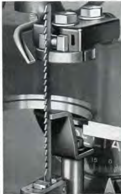
View of the highly efficient disk guide and roller blade support, and the lower blade guide for sabre sawing.
