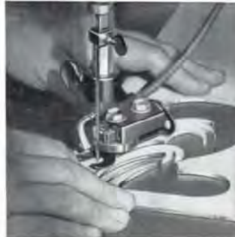
For cutting out intricate designs in sheet metal there is no machine quite as satisfactory as the scroll saw.
