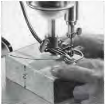
Work up to 2" thick is cut on the Delta scroll saw almost as fast as on the band saw.
