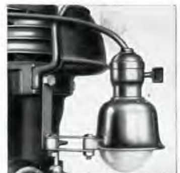
Above is shown the light attachment on the 890 band saw, the neat bracket being typical of newer Delta models. Below, the light attached to an older model drill press, with bracket S-8.
