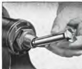
Note, at left, how quickly centers are changed due to the No. 2 Morse taper spindle nose. At right, graduations on tailstock sleeve.
