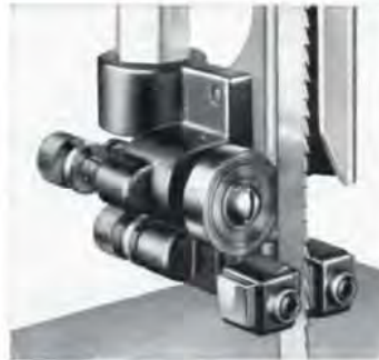
Upper guide, showing ball-bearing blade support and precision adjustments for support and guide pins.
