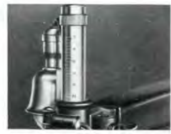
The outer sleeve covering the upper-chuck plunger is moveable and graduated, enabling the user to adjust the tension of the spring to suit his blade, and to return to the same tension at any time.
