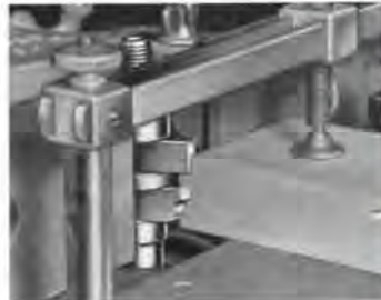
Photo above shows the sliding jig for end-grain shaping from the right side of the machine, showing the stop and pointer on the miter-gage head. Center photo shows how the jig is used on a sash operation, and photo at right how even a short block is shaped safely.
