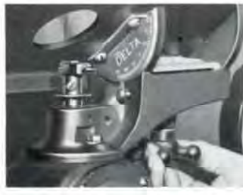
A powerful and convenient hand knob locks the table to the trunnion seats. Table tilts smoothly on heavy trunnions and exact degree of tilt is shown by graduated arc and adjustable pointer.
