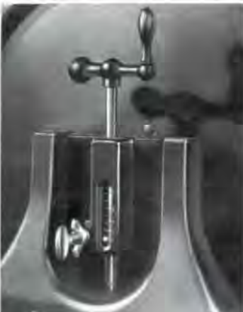
Upper wheel adjustment, with quick index to show blade tension.
