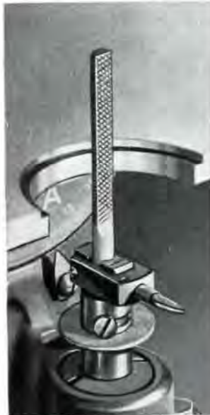
Files, also, are held in the V-jaws of the lower chuck.
