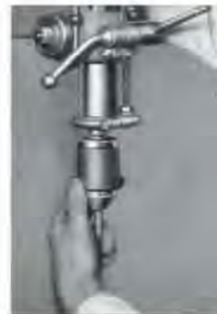
Drills are inserted and removed from Deltagrip chuck with one hand.
