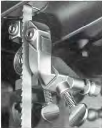
Above and left, two views of lower guide. Note how close to the table the guide pins support the blade.
