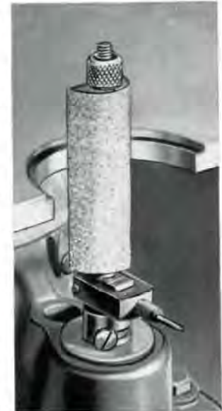
The sanding attachment is held in the V-jaws without any changes.
