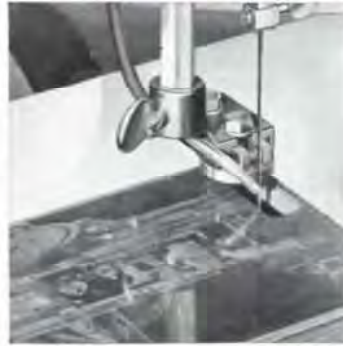
In mortising engravings the scroll saw saves hours of the printer's and engraver's time.
