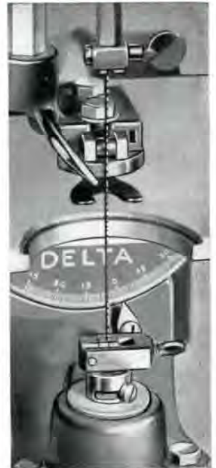
Jeweler's blades are held between the flat saws of the chuck.
