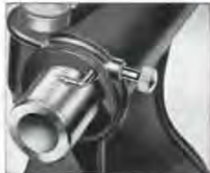
Note, at left, how quickly centers are changed due to the No. 2 Morse taper spindle nose. At right, graduations on tailstock sleeve.
