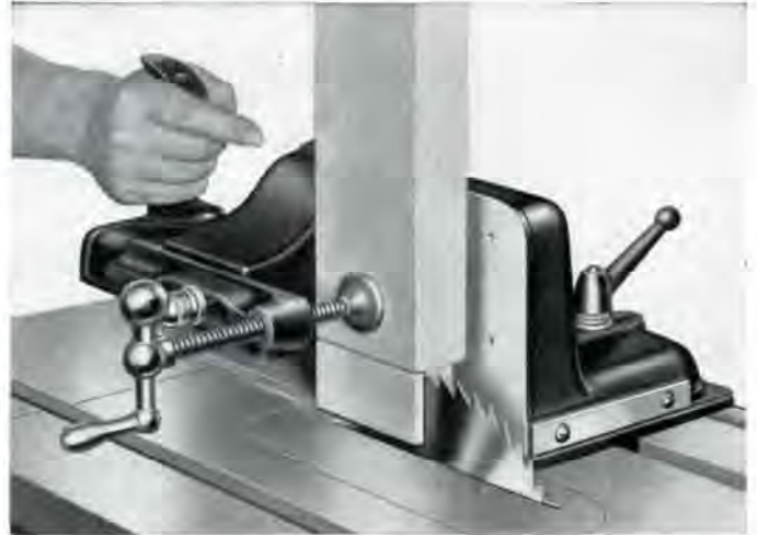
One hand—which never comes near the saw blade—operates this efficient, accurate tenoning jig. Tenoning is now as safe and accurate as any other operation.
