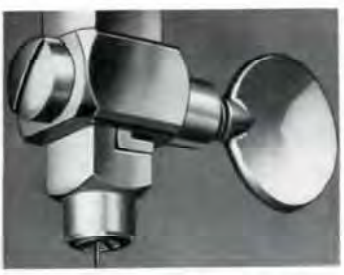
Where very fine blades are used constantly, the self-centering jaw shown here is used in place of one of the regular jaws of the upper chuck. A self-centering lower chuck (extra) is also available.
