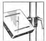
Tilting table (stand-ard) offers every facility for angular work.
