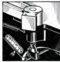
The flap guard can be locked with a padlock to prevent unauthorized removal.
