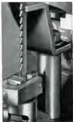
Files, also, are held in the V-jaws of the lower chuck.
