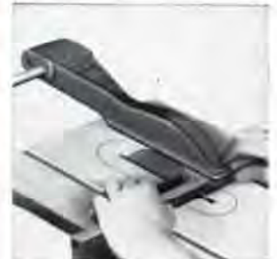
Cutting a steel bar with the abrasive wheel, showing No. 230 Guard in place.
