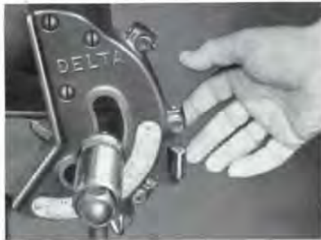
A touch of the finger moves the stop link into or out of engagement. Note the control handle slid out to engage the bracket lock.
