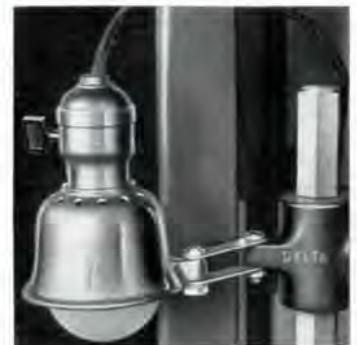
Above is shown the light attachment on the 890 band saw, the neat bracket being typical of newer Delta models. Below, the light attached to an older model drill press, with bracket S-8.
