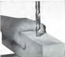
Boring in wood with spur bits is practical because of the standard high speed of the Delta drill press.
