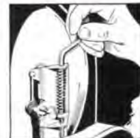
Simple and sturdy wheel-tensioning and tilting device for tracking blade on wheels.
