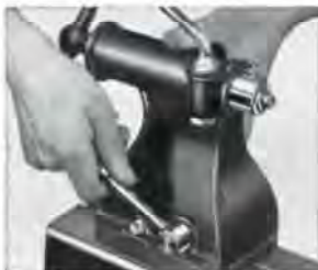
No wrenches required to move the Delta tailstock; a bandy ball-end lever locks and unlocks it.
