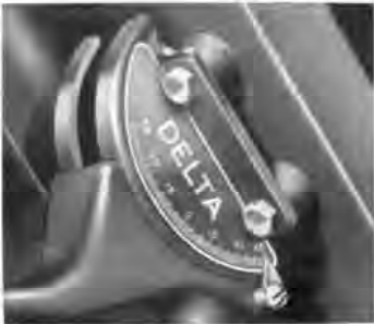
Front trunnion closeup; note graduated index plate and adjustable pointer.
