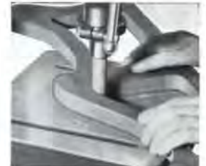
Sanding the edges of carved work with the sanding drum saves hours of tedious labor in the shop.
