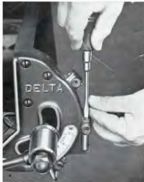
The 45, 90 and 135-degree stops are set with precision. Note the fence handle slid IN to engage the fence tilting lock.
