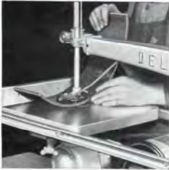
Cutting brake lining is one of the jobs that this scroll saw is performing with satisfaction.
