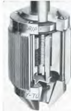
Cut-away view of Deltagrip chuck showing sturdy interior construction.
