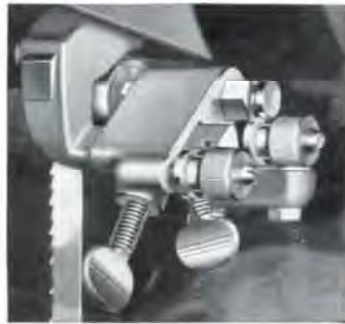
Above and left, two views of lower guide. Note how close to the table the guide pins support the blade.
