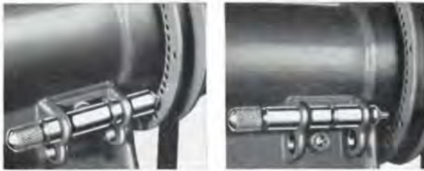
Note double-row index holes: One row, 60 holes, give widest range of divisions: The other row, 30 holes, permits quick indexing of most often used divisions.
