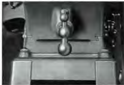
A view of the underside of the table, showing the dovetail ways on which the tables move. Note the gib at the right to permit adjustment for wear.
