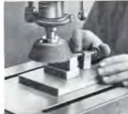
Surface grinding is one of unusual jobs for which this modern tool is adapted, and which it does well.
