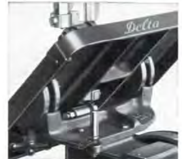
Underside of massive table. Note the heavy steel double trunnions and the removable stop sleeve.
