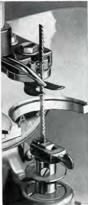
Sabre blades are held in the V-jaws of the lower chuck.
