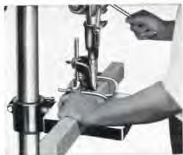
Making a 1/2" mortise on the drill press. Note how the sturdy hold-down keeps the work to the table during the up stroke of the chisel, and how the curved arms hold the work to the fence, allowing the operator's whole attention to be devoted to the accuracy of his work.
