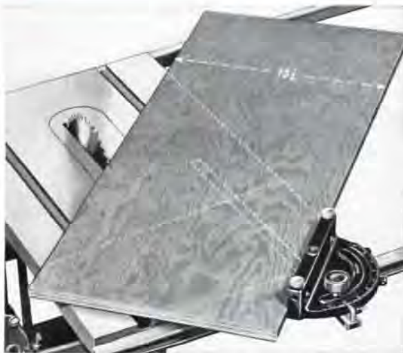
Here is a panel 13 1/2 inches wide being mitered on the Delta Circular Saw with Front Table Extension, a job that would be absolutely impossible to do accurately on the ordinary saw with limited room in front of the saw blade. The dotted lines show how both miter gage and work receive complete support from the table, thus insuring an accurate cut without trouble.
