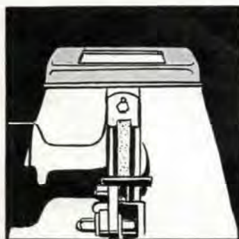
The Lamp Attachment throws a flood of light on the face and on BOTH SIDES of the wheel, making close work easy and fast. (Patent Applied For).
