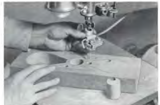
The upper guide is removed in a moment, leaving plenty of room above the blade for the insertion of the blade in interior work, or the removal of heavy work.
