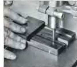
The routing of all kinds of grooves is made absurdly simple, using standard router bits in the special spindle.
