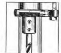
Router spindle takes all spur and other bits with 1/2" shank.
