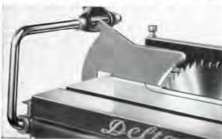
Splitter used alone, without basket guard. At right is shown guard swung completely out of the way.
