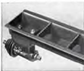
Underside of Delta lathe bed. Crosspieces welded in every 6" makes it tremendously strong.
