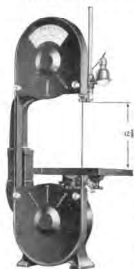
Upper wheel adjustment, with quick index to show blade tension.
