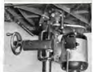
Entire mechanism is one unit assembled and bolted to bottom of table, nothing to get out of alignment, insures true running.
