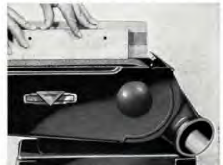
Convenient Wood Fence No. 1410 can be used to support large pieces. Adjustable deflector at end of hood catches dust and carries it off through dust spout. Can be attached to shop dust collecting system.
