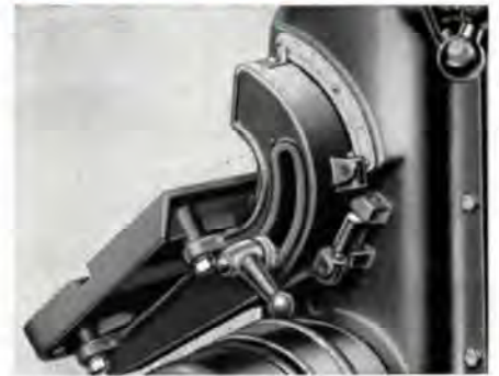
Here's a close-up of the heavy trunnion that carries the tilting table, showing the swinging stop link and adjustable stop screws. A tilting scale and adjustable pointer are also provided.
