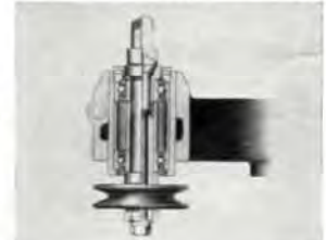
Spindle assembly showing rugged design, short, stiff drive spindle, well spaced bearings . . . produces chatterless work.
