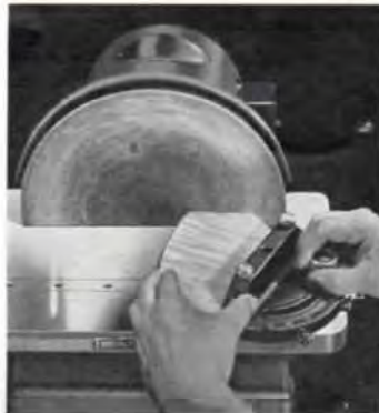
Plain and compound miters are easily handled with the aid of the No. 864 Miter Gage. Accuracy makes it ideal pattern shop tool.
