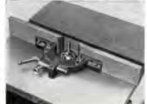
Fully adjustable fence—both halves adjust independently—adjustable endwise so opening may be made small as required.
