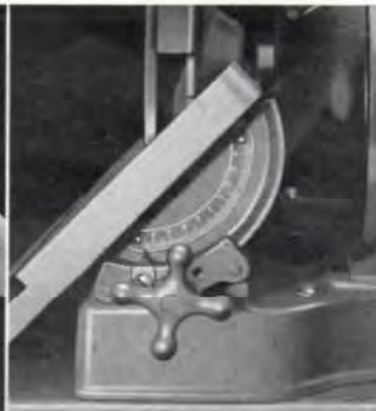
Handy lock knob on either side of table locks it securely at any angle. Scale shows exact degree of tilt.
