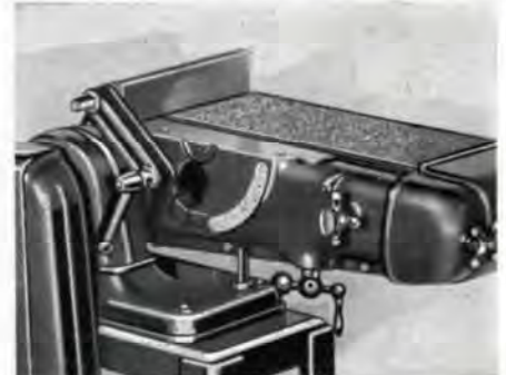
View showing No. 1403 adjustable back stop and its bracket. This is available for use in sanding flat work, to prevent the work from being carried along with the belt.
