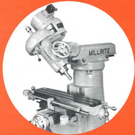
Compound swivel ram permits double angle setting.
