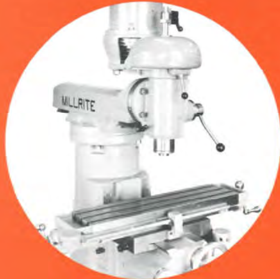
Rapid hand quill feed for production drilling.
